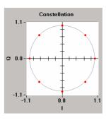
Fig. 3.1: Mapping for 8PSK EDGE.
