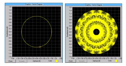
Fig. 3.4: Comparison of a GMSK (left) and an EDGE (right) vector diagram with random data.
