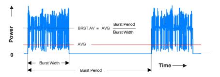
Fig. 2.2: Measuring the average burst power.
