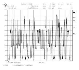
Fig. 3.9: Spectrum analyzer shot of a single EDGE burst with powerramping, here in linear range; the unit is Watt.
