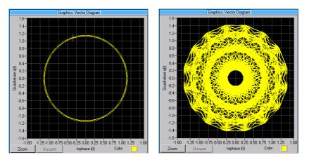
Fig. 3.6: Comparison of two EDGE signals, one with "all 1" data (left), the other with random data.
