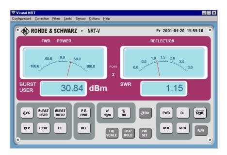
Fig. 8.1: Main panel of Virtual NRT.
