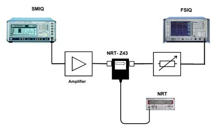
Fig. 2.1: Measurement setup to investigate the power properties of EDGE bursts.
