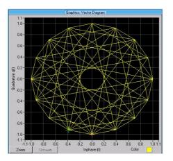
Fig. 3.3: Possible I/Q mapping points for EDGE (including the mapping rotation)
