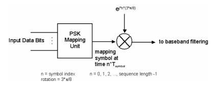
Fig. 3.2: Mapping rotation for EDGE
