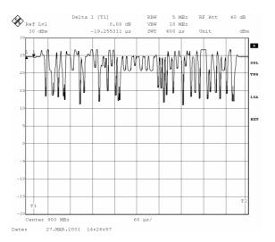
Fig. 3.8: Spectrum analyzer shot of a single EDGE timeslot without powerramping, logarithmic scale. The only "1" data in the guard and tail bit fields lead to a nearly constant power which is higher than the average power in the fields with changing data.
