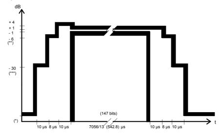
Fig. 5.1: Power time template for GMSK normal burst
